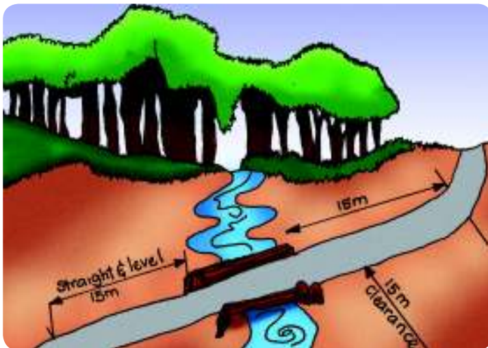
Figure 10.7.1: Roads should be located to avoid steep side cuts and approach stream crossings at right angles where possible.
